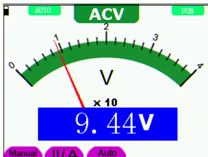
figure 23: AC Voltage Measurement
